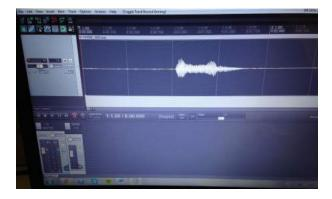
Fig. 7. REAPER Voice Track: Notice the wave that is present. This wave is a graphical representation of my voice saying "Hello". The units of the graph are amplitude over time. Amplitude is in decibels, which is what the human ear interprets as loudness. Time is in seconds.
