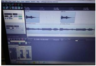
Fig. 14. REAPER Slid Over Vocal Tracks: The two separate parts where "Hello" is said as seen in Figure 13 have merely been shifted over so that they start at the same time that the guitar chord starts.
