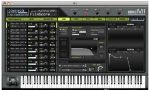
Fig. 19. Korg Keyboard VSTi: Notice the VSTi has keys and controls just like a physical keyboard does. When the keys are set to be played in a sequence and the tone of the keyboard is set to that of a piano, the sound created from this digital keyboard will very accurately simulate the playing of a real piano.
