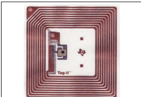
Figure 1 - An RFID Tag, Chips holding data are located in the center, while the antenna used for power and transmission circles the tag.
